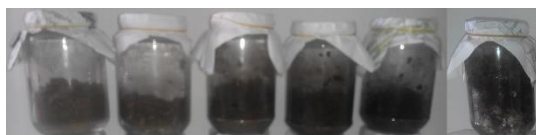
Figure 2. Fermentation in solid media by A. awamori KT 11: (1) rice+ mineral+rice bran, (2) rice+mineral, (3) cassava peel+mineral+rice bran, (4) cassava peel+mineral, (5) cassava peel, (6) rice
